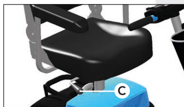
Removing the seat
