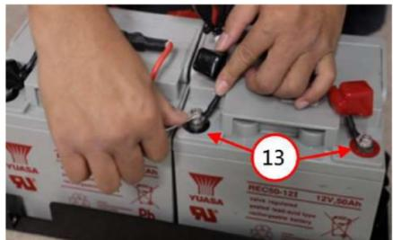
**Step9.2.4** After replacing the battery, perform these steps in reverse order to remount the battery box.
