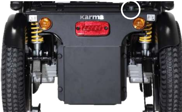
Circuit breaker location
