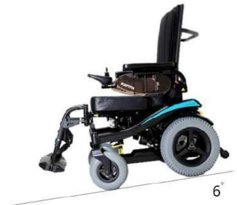
Max. acceptable downhill slope
