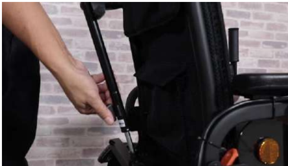
Push the recline lever on Sling Seat
