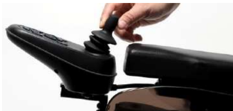
Pull the joystick towards the user
