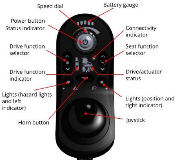
Control Panel with No Tilt & Lighting System Control Panel with Tilt & Lighting System
