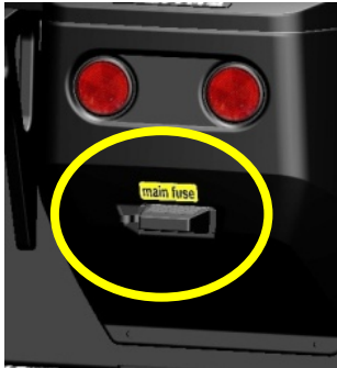
Place of the main fuse
