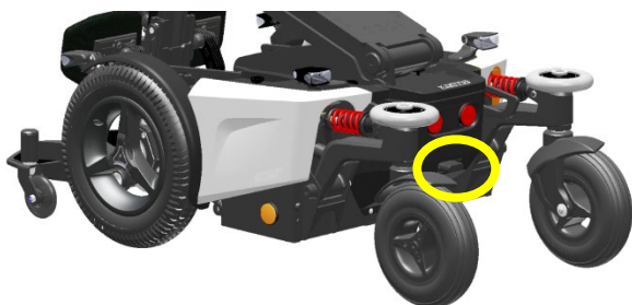
Position main fuse
