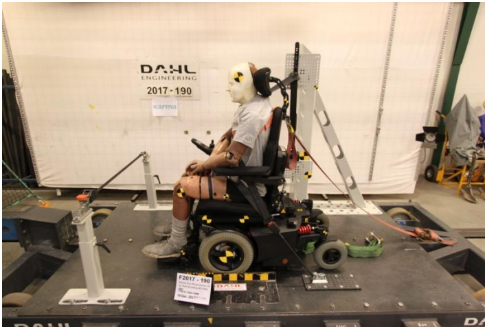
EvO Altus crash test using Dahl Docking station.
