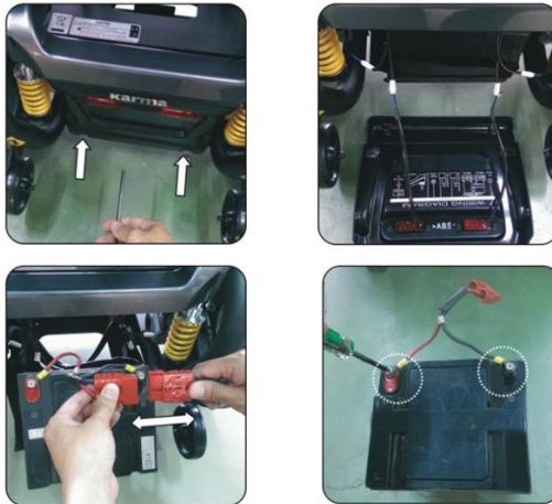
position and access of the maintenance free batteries
