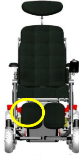
position of the main fuse
