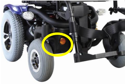
position main fuse
