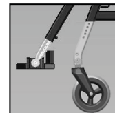
T3-B: 5 holes visible
