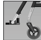
T3-A: 4 holes visible
