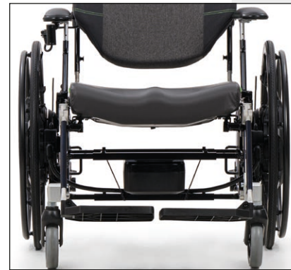
System box (iBox) on the Roxx
