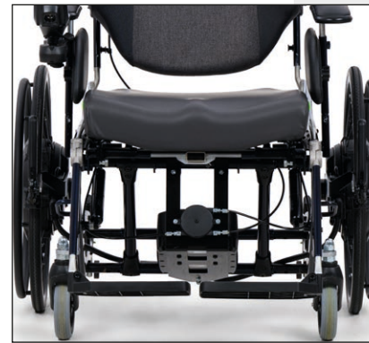
System box (iBox) on the Canto Nxt
